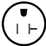
110-120 VAC NEMA 5-20R Single Phase
