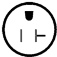
110-120 VAC NEMA 5-20R Single Phase
