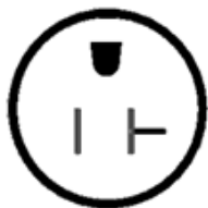
110-120 VAC NEMA 5-20R Single Phase
